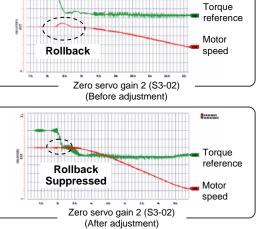
Anti-Rollback with sensors is easy to adjust, preventing shock start and stop.
