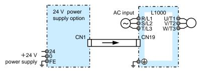
Note: Even if a back-up power supply is used for the control circuit, the main circuit must still have power in order to charge parameter settings.
