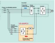
Regenerative Power Supply with RC5 (re-using regenerative energy)
