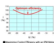
Maximizing Control Efficiency with an IPM Moto (minimizing output current (I) during operation)
